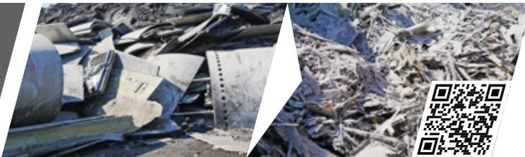
The recycling of CFRP/GFRP materials (the main component of rotor blades) is an important subject for wind turbine operators. After being shredded and subjected to a clean separation process, the glass-fibre reinforced plastics can be recycled sustainably.
