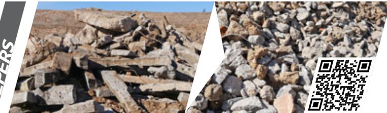
Concrete sleepers play an important role in rail traffic. To ensure the safety of train traffic, they must be replaced regularly. The hard concrete with reinforcing steel is first crushed and the iron content sorted out.
