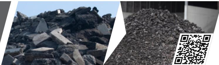
Recycled asphalt is increasingly used in the production of road pavements worldwide. Crushing and screening are followed by processing in asphalt mixing plants. At the end, the processed secondary raw material is reused by road pavers.
