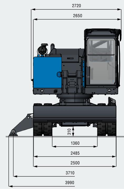
**TRANSPORT DIMENSIONS | TRANSPORTABMESSUNGEN | DIMENSIONS DE TRANSPORT [mm]
