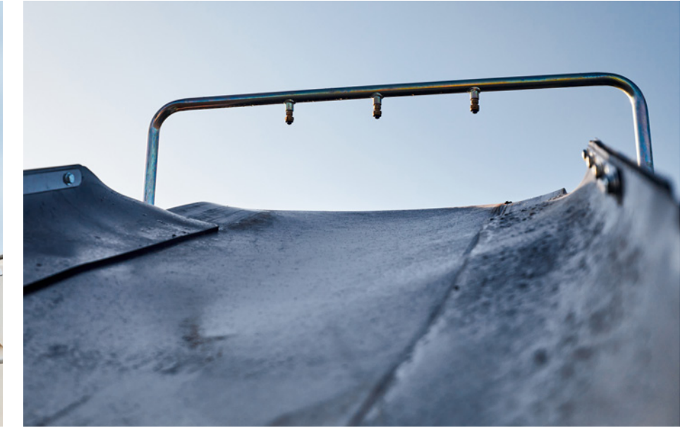
Water spraying system for efficient dust suppression, pump included.
