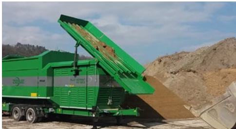
HYDRAULICALLY FOLDABLE STONE GRID (possibility of 4th fraction)
