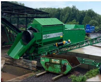
MS 5200-ST with 7 metre long feed hopper and staircase unit.
